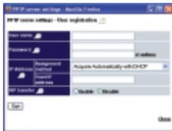
Press the 'Apply' button to register the user. You can register up to 100 users. VPN user status can be seen in the registered user list. An LED on the front of the AirStation (below the WAN LED) will illuminate when a user has initiated a VPN session.
