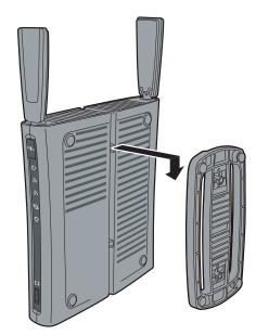
Snap the center of the AirStation to the stand as shown.
