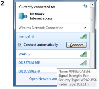
Select the target AirStation and click [Connect]. If you will be connecting to this device in the future, checking [Connect automatically] is recommended.
