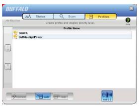
Click the *Profiles* tab to open this page. Use this page to access your profiles. Profiles allow you to save the information associated with a specific wireless network so you can quickly and easily connect to that network when you are in that location. The Profiles page allows you to add, delete, and edit your profiles, as well as import and export data.
