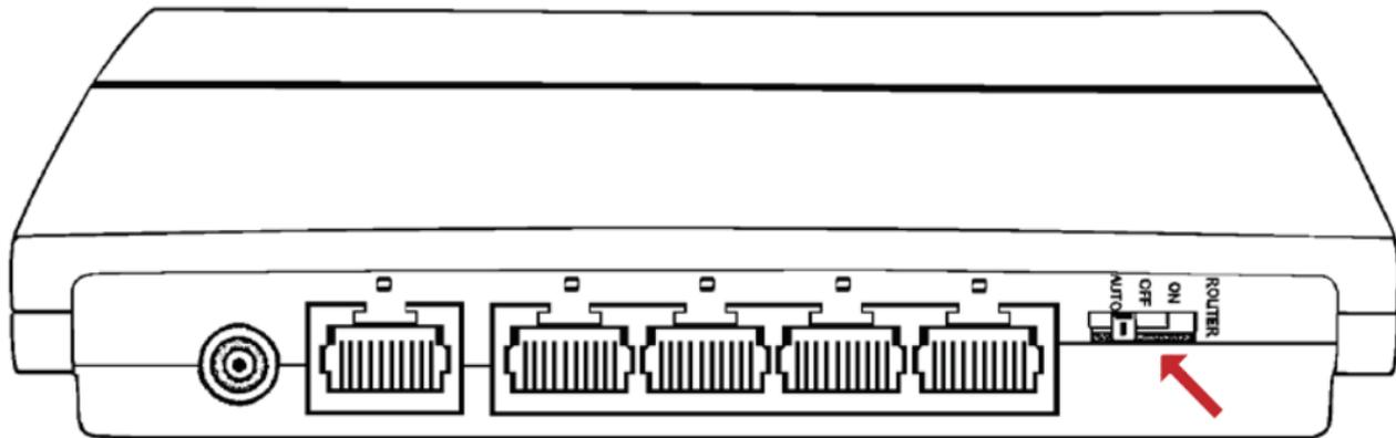
The AirStation may be used as either a full wireless router or a simple access point. The switch has three positions:
