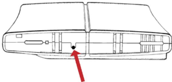
You may also initialize your AirStation by holding down the *Reset* button on the bottom for 3 seconds with a straightened-out paper-clip or similar object.
