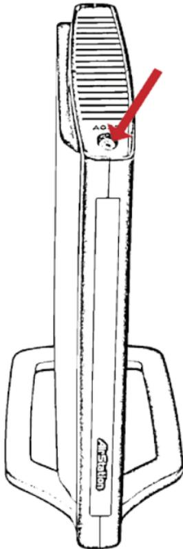
**AOSS** (AirStation One-Touch Secure System) is a simple system for configuring your wireless network securely. If your router and your client device are installed and both support AOSS, then making a secure wireless connection between them is very easy.
