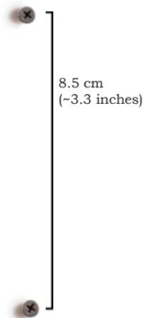
Or, the base can be attached directly to the wall with two screws 8.5 cm (~3.3") apart. After the base is firmly secured, attach the AirStation to its base normally.
