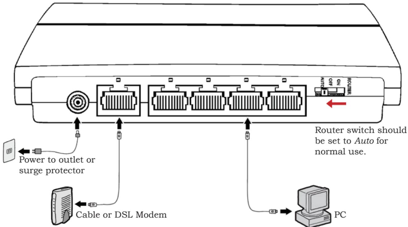
To initially configure your AirStation, you'll use a wired connection to your computer. Once you've connected to the internet through the router, you may switch to a wireless connection if desired.
