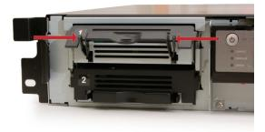
Squeeze the tabs gently and swing the tray latch upward.
