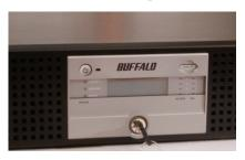
Pull on the right hand side of the front panel to remove it.
