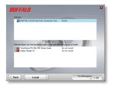
Once the TeraStation is installed, you'll need to install the iSCSI connection tool. Click *Next*, then continue to click *Next*, stepping through the menus until the iSCSI connection tool is installed.
