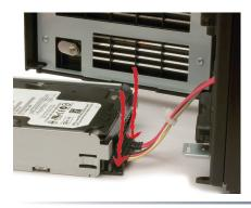
Gently push down on the two tabs to release the plug.
