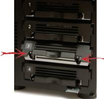
Squeeze the tabs gently and swing the tray latch upward.
