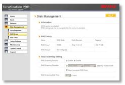
You may also disable *RAID Array Error Detection Response* from this page. Normally, this is set to automatically shut down the RAID array when an error is detected. Though it is not recommended, you may disable that behavior by selecting *Disable*.
