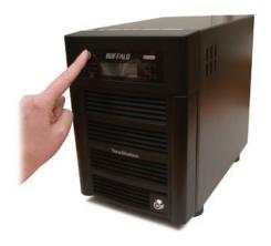
Press the *power button* on the front panel. LEDs will light as your TeraStation boots up.
