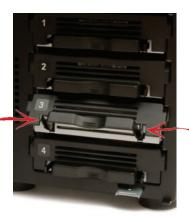
Squeeze the tabs gently and swing the tray latch upward.
