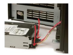
Gently push down on the two tabs to release the plug.
