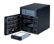
Slide the new drive into the empty drive slot.
