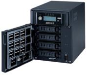
Push the lock tab gently to the left and swing out the drive lock.
