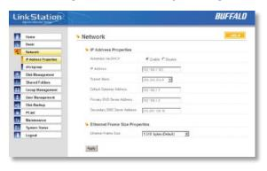
In most networks, LinkStation will get its IP Address automatically from a DHCP server. You may disable DHCP here. If DHCP is disabled and an IP Address is not set manually, it will default to 192.168.xxx.xxx with subnet mask 255.255.0.0. The LinkStation's IP Address, Subnet Mask, Default Gateway Address, and DNS Server address may all be entered manually under IP Address Properties.
