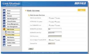
WebAccess is set up from within the Configuration GUI. First, select 'Web Access', and then 'Service Setup' from the menu on the left.
