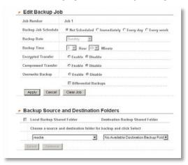
A Backup Job can run regularly on a daily or weekly schedule, or immediately by appropriate choices in the Backup Job Schedule field. Date and Time for the backup may be entered, and Encryption and Compression enabled or disabled. Enable Overwrite Backup to have each scheduled backup write over the previous backup, or Differential Backups to backup only files changed since the previous backup.
