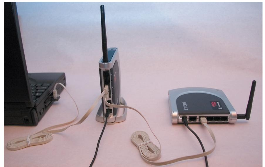
\* Note: Each AirStation may be part of 6 different bridges. Remember that each layer of bridges takes about half your total network speed, so avoid configuring daisy-chains more than 4 bridges long. A star-pattern is always better, with a central router serving multiple bridges.
