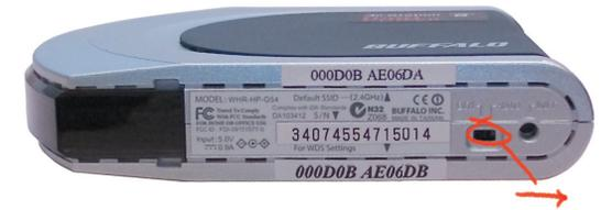
The second AirStation will be configured as a repeater/bridge. Make sure that its switch is set to "BRI". Use a RJ-45 cat5 Ethernet cable to connect LAN ports of the two AirStations. Power up the second AirStation. Connect a PC's Ethernet port to another RJ-45 port on the main router (the first AirStation). You will use this PC to configure the settings of the AirStations.
