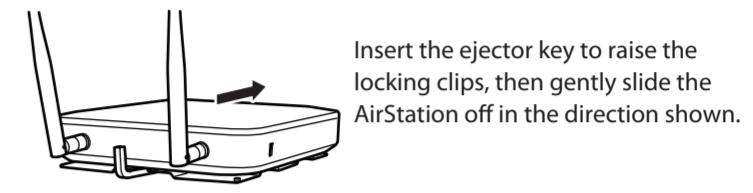
Insert the ejector key to raise the locking clips, then gently slide the AirStation off in the direction shown.
